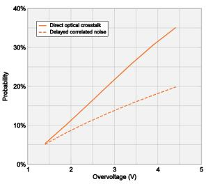
**Fig.9** Correlated noise probability in RGB-SiPMs as a function of overvoltage. Delayed correlated noise includes delayed crosstalk and afterpulse.
