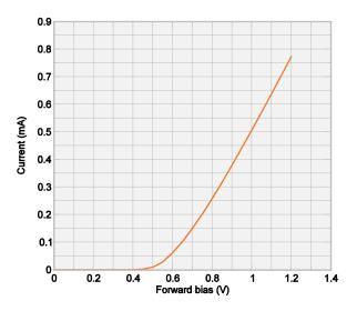
Fig.2 Typical forward IV curve (ASD-RGB1S-P).
