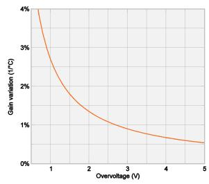
**Fig.6** Relative variation of gain with temperature in RGB-SiPMs as a function of overvoltage.
