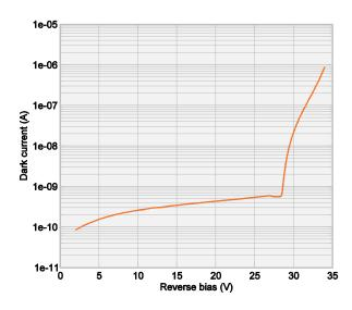
Fig.1 Typical reverse IV curve (ASD-RGB1S-P).
