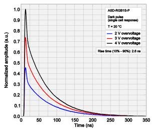
Fig.10 RGB-SiPM pulse shape (dark pulses, single cell response) at different overvoltage. Recharge time constant is 50 ns. Signals acquired with ASD-EP-EB-N.
