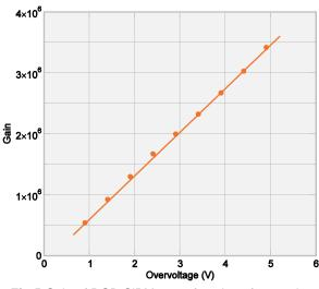
Fig.5 Gain of RGB-SiPMs as a function of overvoltage.
