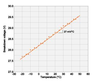
**Fig.3** RGB-SiPMs breakdown voltage temperature dependence.
